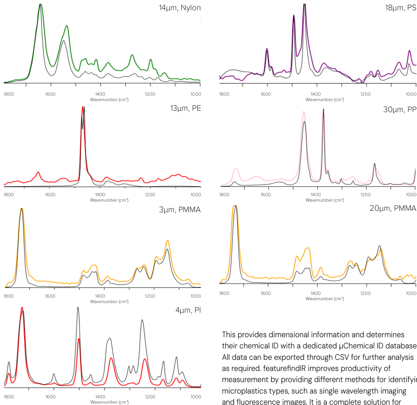
Figure 6: IR spectra overlaid in reference library spectra (black), showing excellent agreement, across all size ranges and plastic types
