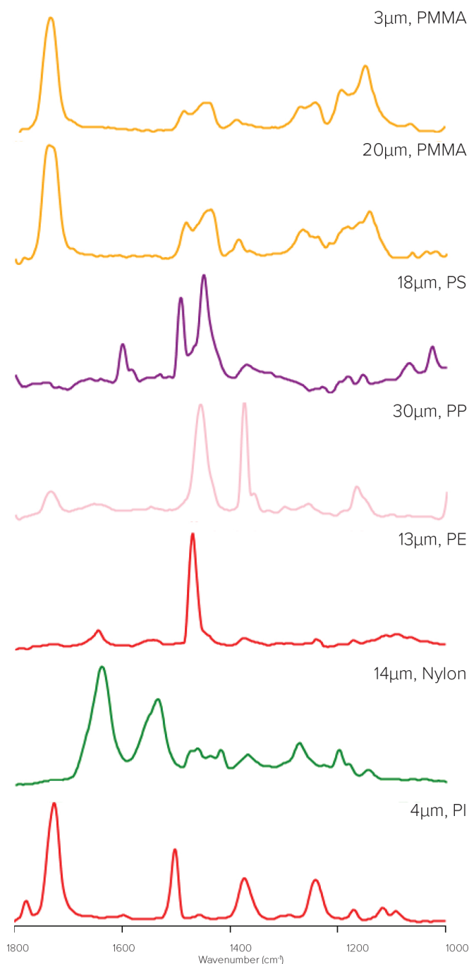
Figure 5: Stacked representative, IR spectra across a wide range of typical microplastics and across a wide range of particle sizes, spanning the challenging <30 \mu m range. Of note is that even articles of 3 \mu m and 30 \mu m from the same material show virtually identical IR spectra.
